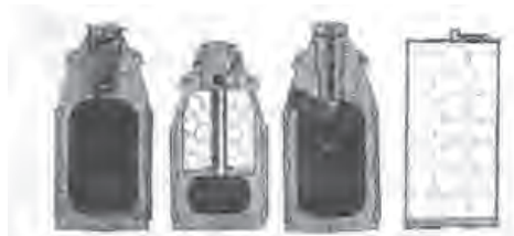
C/61 Ammunition. Pictured are nose fuze Common shell, Schrapnel, Timed fuze explosive, and Case shot.
